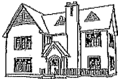
Multiple gambrel roofs appropriate to the Tudor style.
