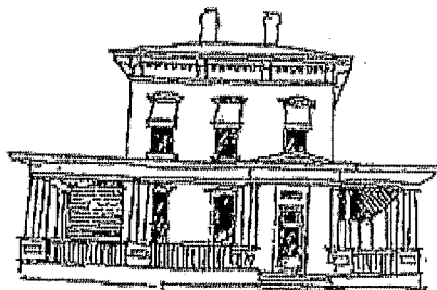
Inappropriately scaled covered porch and architectural style.
